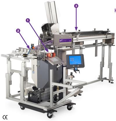
250 ip3 Automatic Feeder Bagging system with APL
