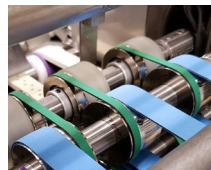
Updated Bridge Belt Assembly (green belts)
